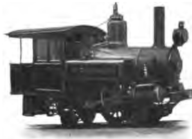
RACK LOCOMOTIVE, RIGGENBACH SYSTEM.
