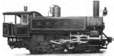
RACK LOCOMOTIVE, WITH TWO COG-WHEELS.
