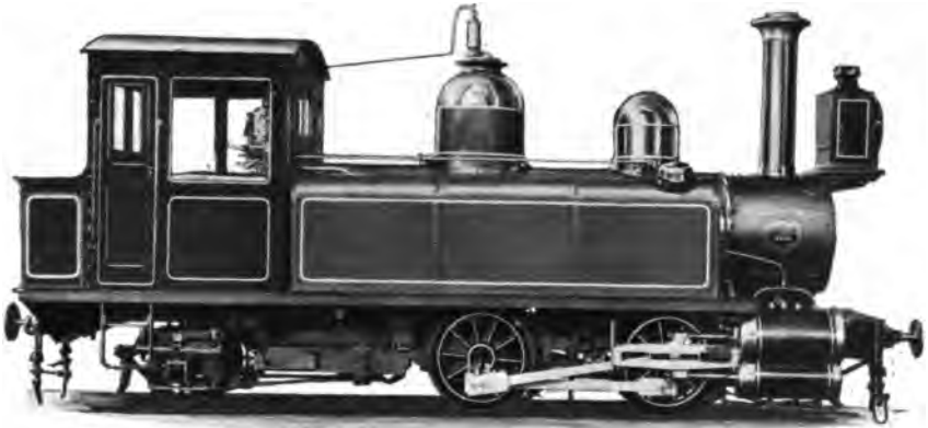
FOUR-COUPLED SIX-WHEEL TANK LOCOMOTIVE STATE TRANSCAUCASIAN.
