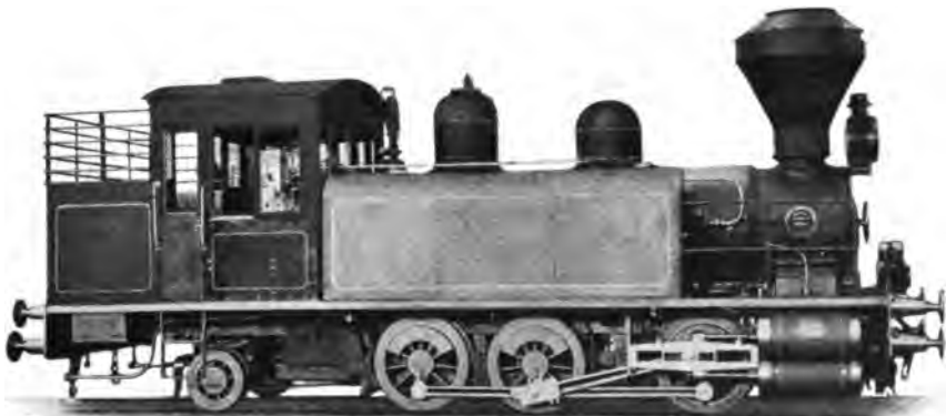
SIX-COUPLED TANK LOCOMOTIVE CHINESE EASTERN RAILWAY
