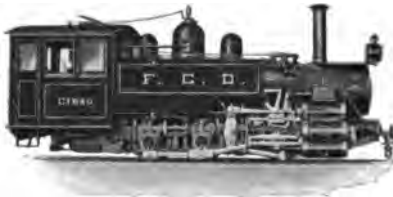
COMBINATION RACK AND ADHESION LOCOMOTIVE.
