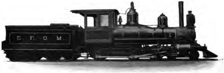
NARROW-GAUGE TEN-WHEEL LOCOMOTIVE, OESTE DE MINAS RAILWAY, BRAZIL.
