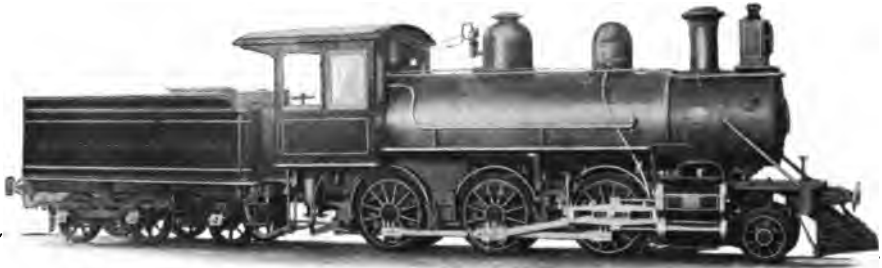
NARROW-GAUGE MOGUL FREIGHT LOCOMOTIVE TIKUHO RAILWAY, JAPAN.
