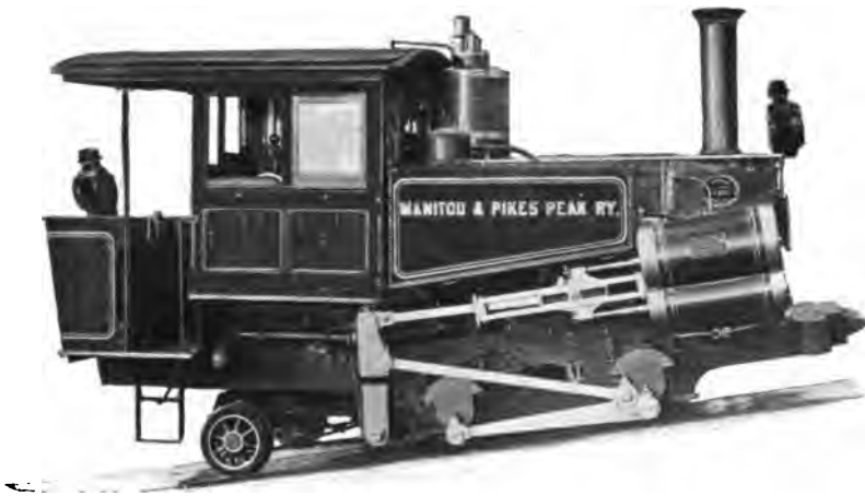
RACK LOCOMOTIVE, MANITOU AND PIKES PEAK RAILWAY.
