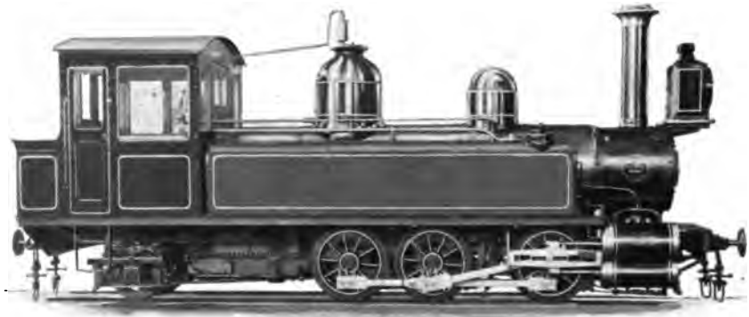
NARROW-GAUGE SIX-COUPLED TANK LOCOMOTIVE, STATE TRANSCAUCASIAN RAILWAY OF RUSSIA.
