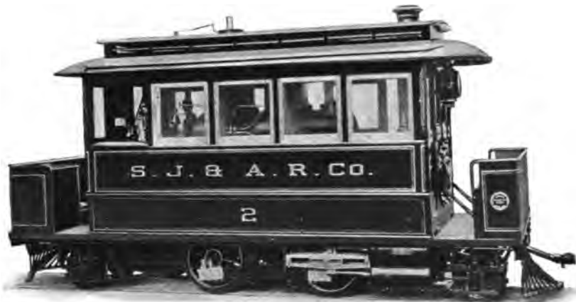
NARROW-GAUGE FOUR-COUPLED DOUBLE-ENDED ENCLOSED LOCOMOTIVE, SAN JOSÉ & ALUM ROCK RAILWAY.
