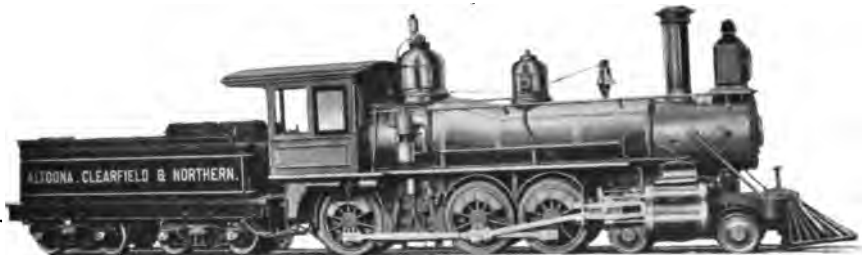
TEN-WHEEL PASSENGER LOCOMOTIVE, ALTOONA CLEARFIELD & NORTHERN RAILROAD.
