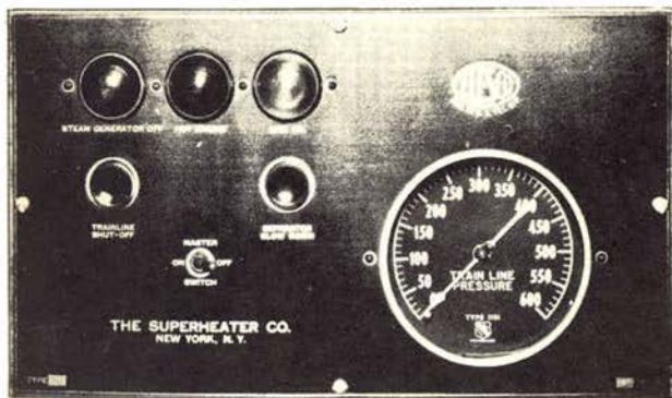
Fig. 6-3 - Remote Control Panel
