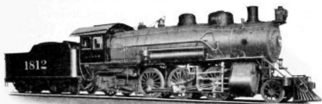
BALANCED COMPOUND PRAIRIE TYPE LOCOMOTIVE For the Atchison, Topeka & Santa Fe Railway
