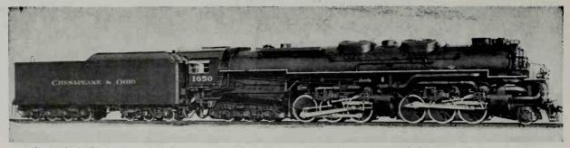
Chesapeake & Ohio 2-6-6-6 Type Single-Expansion Articulated Locomative, Class H-8, Nos. 1600-1644 built in 1941 and 1645-1659 in 1949.
