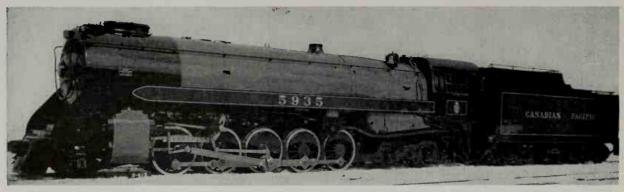
Canadian Pacific 2-10-4 Type Locomotive, Class T-1c, No. 5735, for freight service, Nos. 5930-5935. Equipped with Booster. Built by the Montreal Locomotive Works, Ltd. in 1949.
