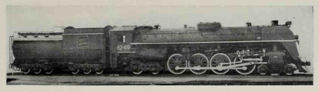
Canodian National 4-8-4 Type Locomotive for passenger and fast freight service, Class U-2h, Nos. 6235-6264. Built by the Montreal Locomotive Works in 1943 and 1944.
