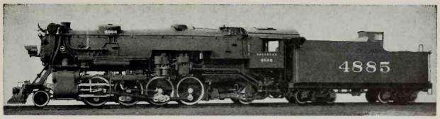
Southern Railway 2-8-2 (Mikado) Type Locomotive for freight service, Nos. 4885-4914. Built by The Boldwin Locomotive Works in 1928
