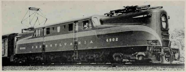
Pennsylvania Railroad 11,000-Valt Alternating Current Locomotive, Class GG-1, Nos. 4800-4938, for passenger service, built by General Electric Company, Westinghouse Electric Corporation, The Baldwin Locomotive Works and Pennsylvania Railroad.
