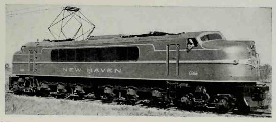
New York, New Hoven & Hartford Electric Passenger Locomotive, Class EP-4, Road Nos. 0361-0366, combination 11,000-volt A.C. overhead and 600-volt D.C. third rail, built by General Electric Co. in 1938.
