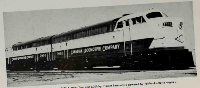
Canadian Locomotive Compony, Ltd. No. 7005 & 7006, Two Unit 3,200-hp. Freight Locomotive powered by Fairbanks-Morse engines.
