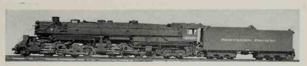
Northern Pacific 2-8-8-4 (Yellowstone) Type Locomotive, Class Z-5, Nos. 5001-5011, Built by The Baldwin Locomotive Works in 1930.
