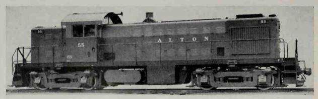
Alton No. 55, Class DSA; 1,000-Hp. Road Switching Locomotive built by American Locomotive Company-General Electric Company in Nov. 1945.
