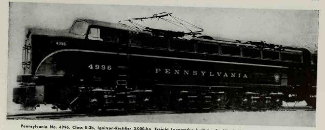
Pennsylvania No. 4996, Class E-3b, Ignitron-Rectifier 3,000-hp. Freight Locomotive built by the Westinghouse Electric Corp., in 1951.
