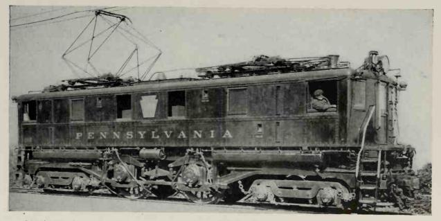
Pennsylvania Railroad 11,000-volt Alternating Current Locamative, No. 7850, Class O-1, for passenger service, built at Altoona in 1930.
