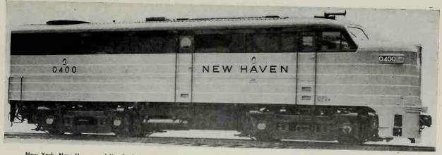
New York, New Haven and Hartford No. 0400; 1,500-Hp. Diesel-Electric Freight Locomotive, A Unit built by Alco-G.E. in May 1947.
