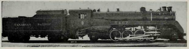
Canadian Pacific 2-8-2 (Mikado) Type Locomotive, Class P2k, Nos. 5462-5473. (Four coal burners, eight oil burners). Built by the Montreal
