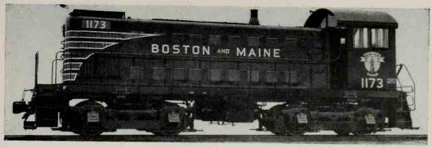
Boston & Maine No. 1173; 660 Hp. Switching Locomotive built by Alco-G.E. in September 1950.
