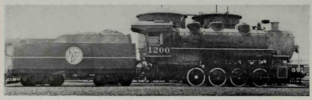
Atlantic Coast Line 0-8-0 (Eight-Wheel) Switching Locomotive, Class E-14, Nos. 1200-1234. Built by The Baldwin Locomotive Works in 1923-1926.
