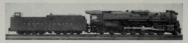
Pennsylvania Railroad 2-10-4 Type Locomotive, Class J-1, No. 6474. Built by the Pennsylvania Railroad Company in 1942, 1943 and 1944.
