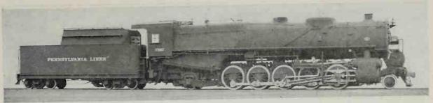
Pennsylvania 2-10-2 (Santa Fe) Type Locomotive for freight service, Class N-1-s, No. 7227. Built at the Brooks Works of the American Locomotive Co. for the Pennsylvania Lines in 1918.
