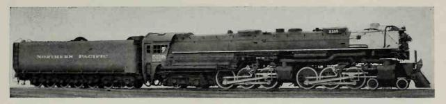
Northern Pacific 4-6-6-4 Type Single-Expansion Articulated Locomotive for freight service, Class Z-8, Nos. 5130-5149. Built by the American Locomotive Company in 1943 and 1944.
