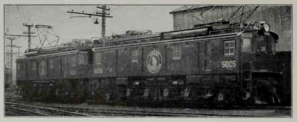
Great Northern Double-Unit Motor-Generator Type Electric Passenger and Freight Locamotive, Class Z-1, built by The Baldwin Locamotive Works and Westinghouse Electric Corporation in 1926.
