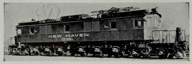
New York, New Haven & Hartford 11,000-volt A.C. and 600-volt D.C. Electric Passenger Locamative, Class EP-3, Road Nos. 0351-0360, built by
