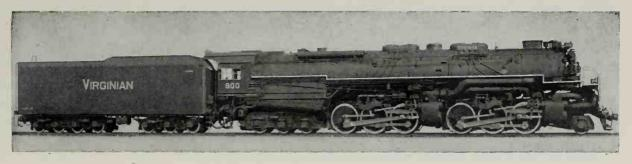
Virginion 2-6-6-6 Type Single-Expansion Articulated Locomotive: Class AG. Nos. 900-907. Built by the Lima Locomotive Works. Inc. in 1945.
