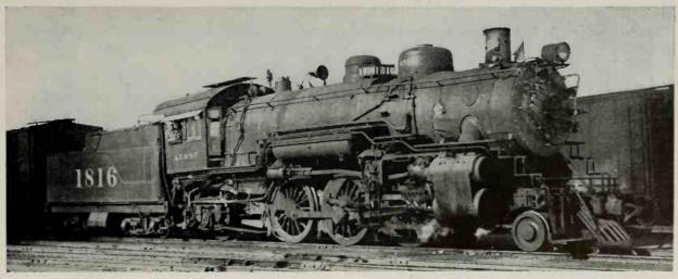
Atchison, Topeka & Santa Fe 2-6-2 (Prairie) Type Locomotive for freight service No. 1816. Built by The Boldwin Locomotive Works in 1906. Rebuilt by the A. T. & S. F. in 1928.
