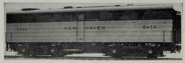
New York, New Haven and Hartford No. 0450; 1,500-Hp. Diesel-Electric Freight Locomotive, B Unit built by Alco-G.E. in May 1947.
