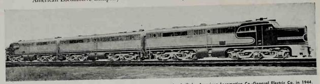
Atchison, Topeka & Santa Fe No. 51, Three Unit 6,000-Hp. Passenger Locomotive built by American Locomotive Co.-General Electric Co. in 1944.
