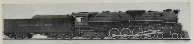
Chesapeake & Ohia 4-8-4 Type Locomotive for passenger service, Class J-3a, Nos. 605-606 and 610-614. Built by Lima Locomotive Works, Inc. in 1948.
