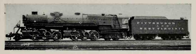
Pittsburgh & West Virginia 2-6-6-4 Type Single-Expansion Articulated Locomotive, Nos. 1100-1102 and 1103-1106. Built by The Baldwin Locomotive Works in 1934-1937.
