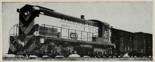
Chicago & North Western No. 1502, Baldwin-Westinghouse 1,600-hp. All-Service Locomotive with six axles and six motors, Model AS-616.
