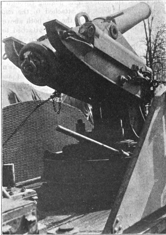
155-MM. HOWITZER MOUNT. WORKING PLATFORMS IN TRAVELING POSITION.
