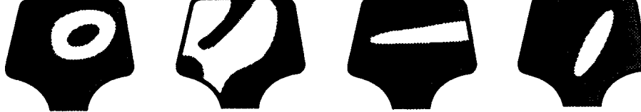
A Transverse Fissure B Compound Fissure C Horizontal Split Head D Vertical Split Head
