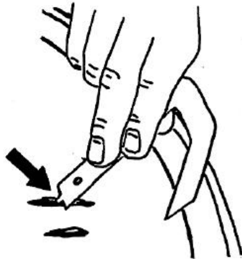
Figure A-5. Gauging defective wheels.
