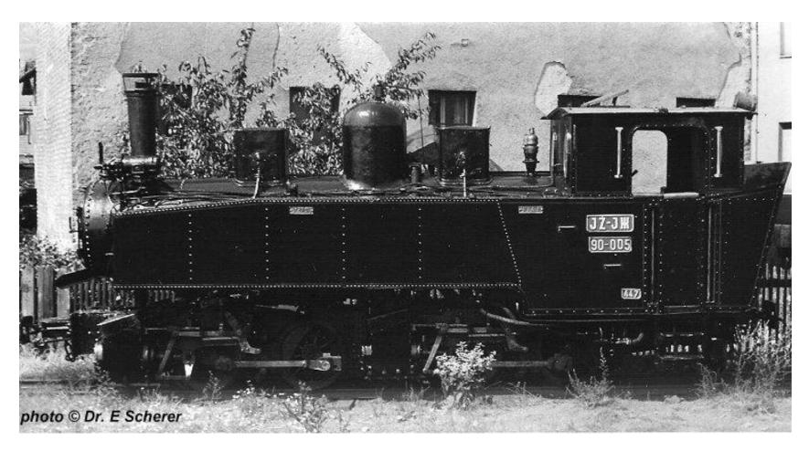
0-4-4-0 90-005 is seen in ex-works condition at Sarajevo during August 1965. This loco was built by Hohenzollern in 1911
