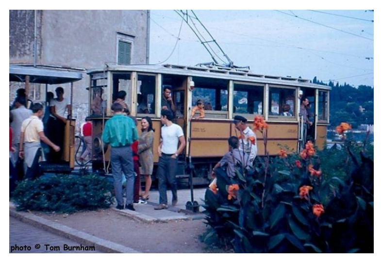
Tom Burnham writes: a small system of 760mm gauge, with a Y-shaped layout - this is at the junction (see point lever in front of the tram). There were two versions of the 4-wheeled trams, one with a slightly more modern styling, running in motor-trailer sets. The afternoons tended to see power cuts, and the trams would regularly come to a dead stop along the Put Marsala Tita.
