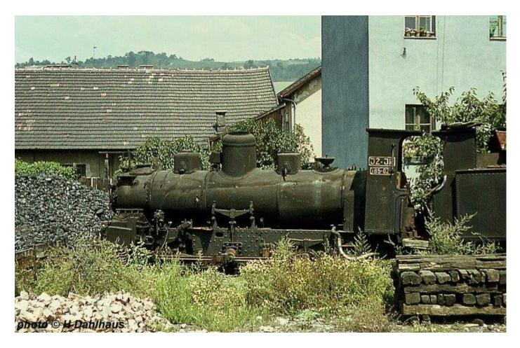
The sad remains of 185-023 (Arad 110/1901), a Klose system 0-6+4 tender loco. Altogether Krauss in Linz and Weitzer in Arad built 45 of this class. Between the wars some machines had the Klose mechanism removed. 11th August 1966.
