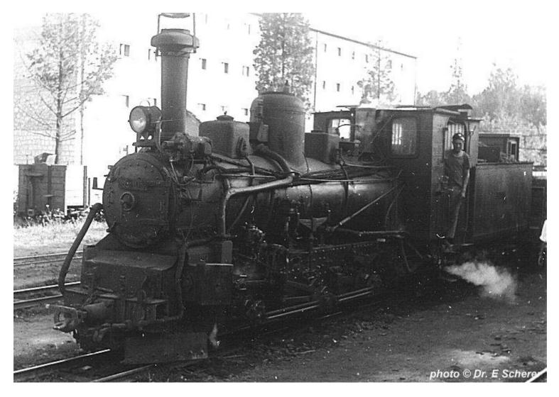
185-025 at Capljina in August 1965. 41 examples of this class of 0-6+4 tender locomotives were built between 1900 and 1901. This one has had its Klose mechanism removed.
