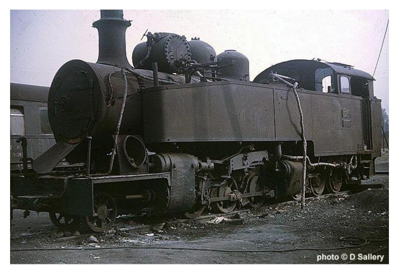
This loco was in use in 1967 as a stationary boiler at Sarajevo Novo - the new standard gauge station. It is a 2-6-6-0 compound tank No. 91-021. A total of 38 were built by Henschel. All have since been scrapped. These locos were all out of use in the 1950's and this could have been the last survivor. The size and sophistication of the loco gives an indication that the narrow gauge was very much a main line operation.
