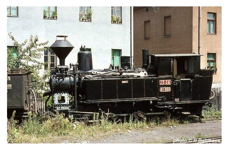
Newly overhauled 81-006, an 0-8-0 tank built in Budapest in 1914, waits to return to its home depot of Zavidovici. This loco was built with Klien Lindner axles and was identical to the Budapest/MAVAG type 70 which was built between 1905 and 1950. A total of 142 were built and they were also found in Romania. 11th August 1966.
