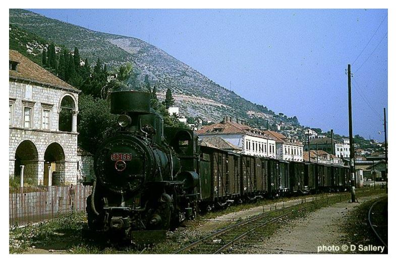
No. 83-166 has finished marshalling its train and is ready to leave Dubrovnik on an afternoon freight. The bogie goods vans were quite large vehicles for the 76cm gauge.
