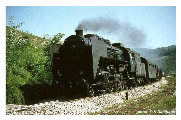
With the 76cm line on the right this is 4-8-0 11-054 (MAVAG 7413/1955) with a goods train from Sarajevo at Semizovac on 11th August 1966. These impressive locos were identical to the Hungarian class 424 and a total of 63 were built for service in Yugoslavia.
