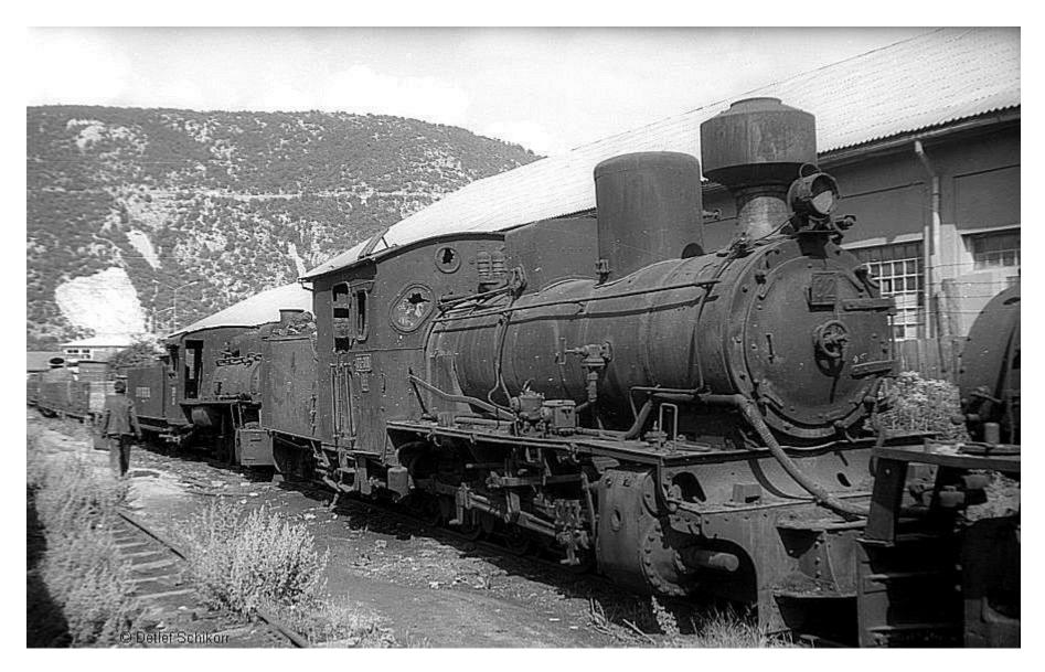
JZ 32, a superheated 0-10-0 built in 1924 on shed at Drvar 12.8.1970. No. 32 was one of a series of four, Nos. 29 to 32, built by Orenstein & Koppel.
